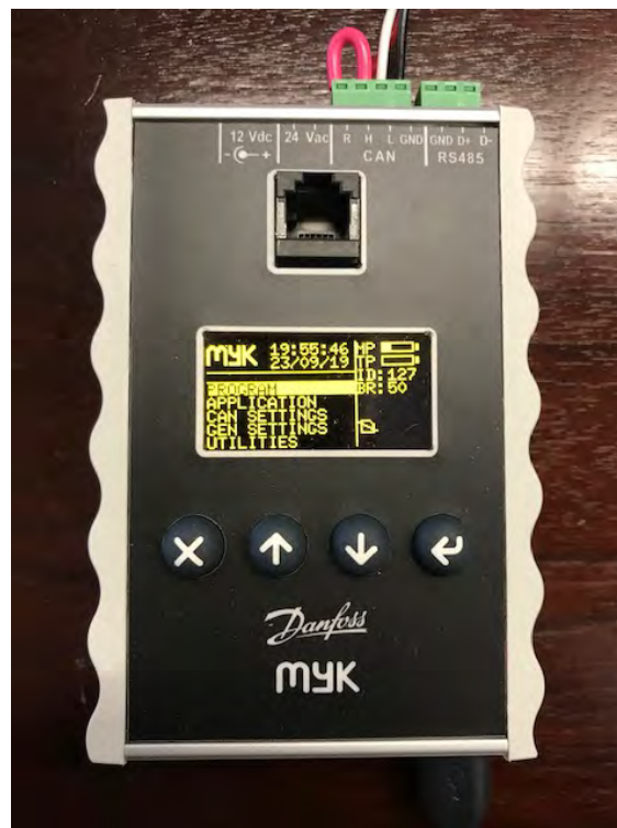
Figure 52 MMIMYK CONNECTIONS - CANBUS TO MCX06D
