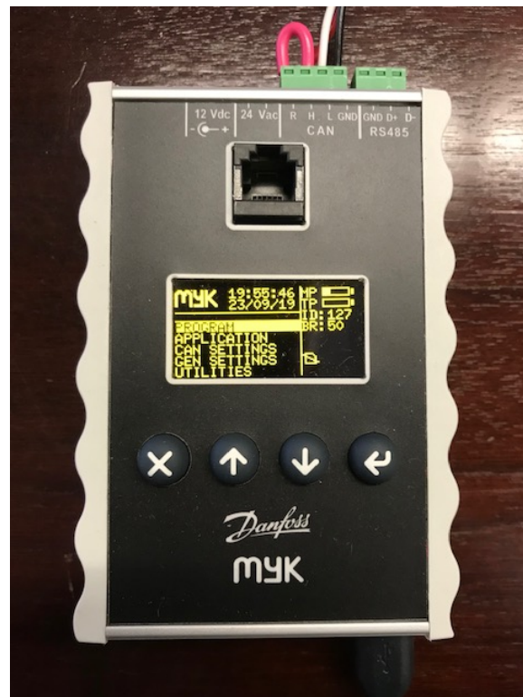
Figure 47 MMIMYK CONNECTIONS - CANBUS TO MCX06D
