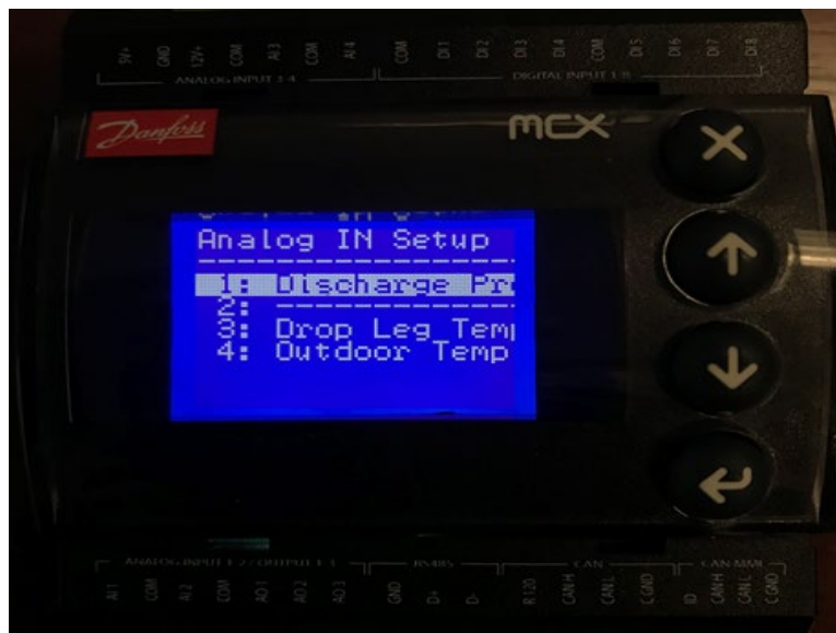
Figure 61 ANALOG INPUT SETUP SCREEN
