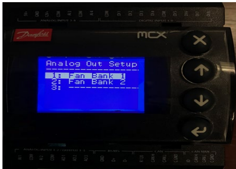
Figure 63 ANALOG OUTPUT SETUP SCREEN
