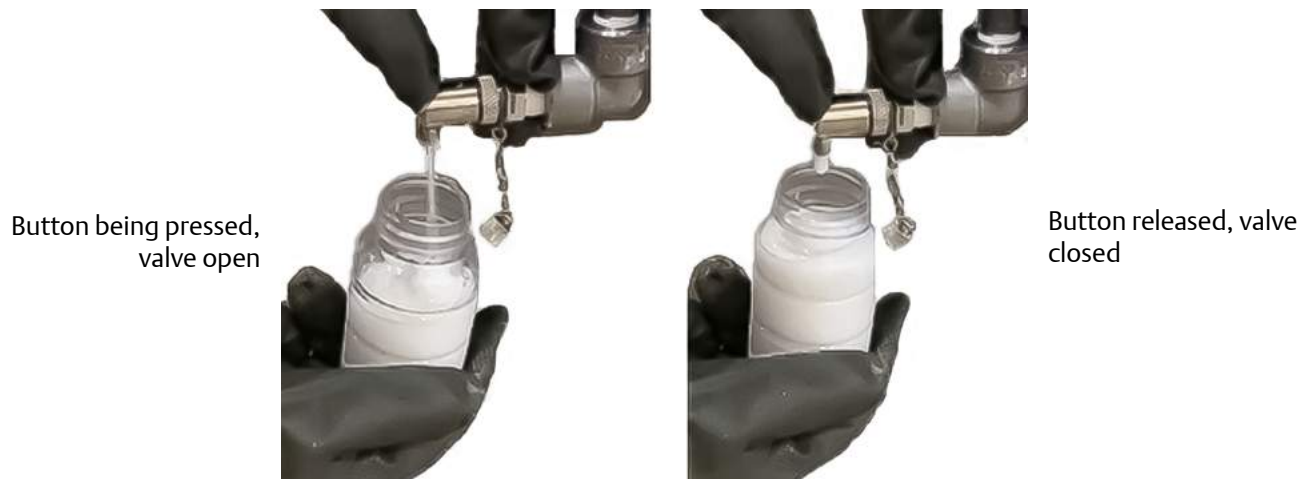
Figure 5-5. Operating the Oil Sampling Valve
